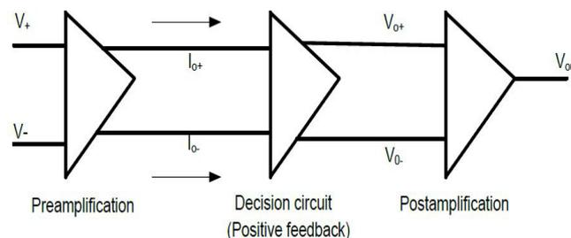
Figure 1(c): Block diagram of Comparator
