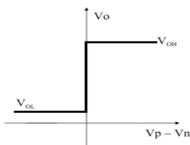
Figure 1 (b): Ideal voltage transfer characteristic of comparator.
