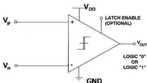
Figure 1 (a): Schematic of Comparator
