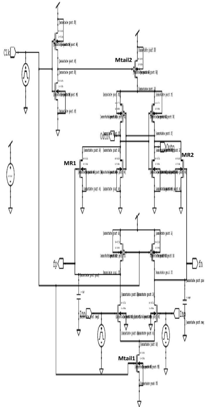
Figure 2 (b): Schematic of the Conventional Double Tail Comparator
