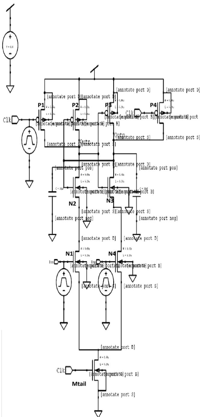
Figure 2 (a): Schematic of the Conventional Comparator
